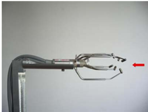
Figure 4 - Ultrasonic Anemometer sensing element; the arrow indicates the flow direction
