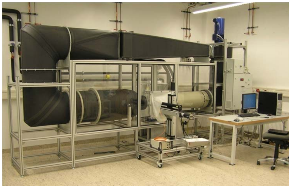
Figure 1 - Closed loop wind tunnel with an open test section
